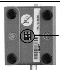
Remove the silver tape to expose the DIP Switch Bank under the unit
